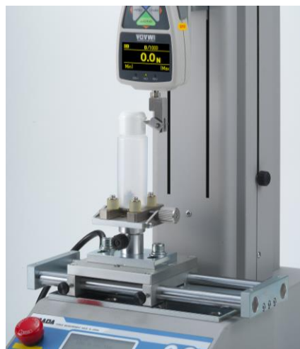
HFC-50N Testing Image (Flip Cap Opening Force Test)
