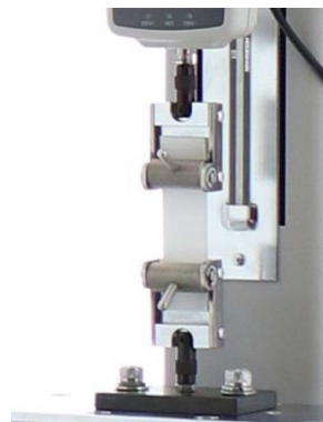
Test Image (Tensile test of paper)
