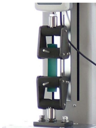
Test Image (Tensile test of rubber sheet)
