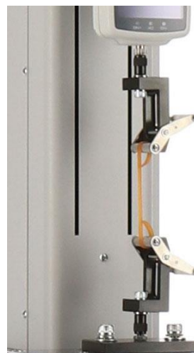
Test Image (GC-60: Rubber tape tensile test)
