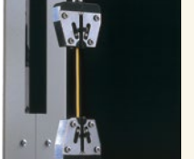
Cable tension strength test with KC-1001.
