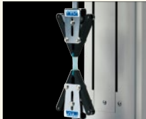
Rubber tension strength test with PGC-0510.
