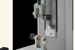
Tensile test of copper wire with WG-1000N
