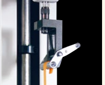
Rubber tape tension strength test with GC-60.
