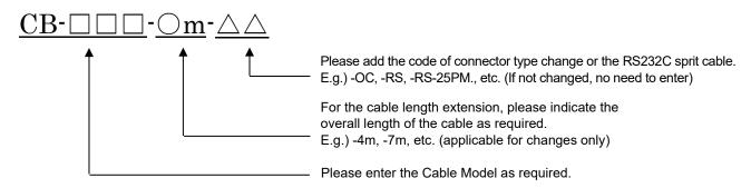
E.g.) Cable Model: CB-108, Overall Length 7m (extended additionally by 4m)  $\rightarrow$  Connector Code : CB-108-7m-BNC
