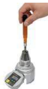
BMRD torque checking with BTGE-G.
