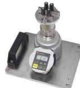
BTGE-G with table attachment and measurement stand
