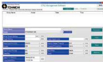
Single spindle tightening mode setting display
