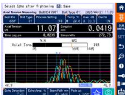
Waveform before & after giving loading
