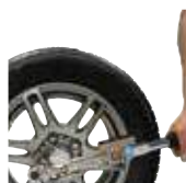
Completion of tightening process with Blue signal.
