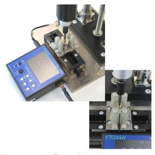
\*Usage example Screw tightening
