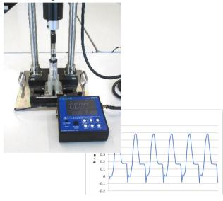
\*Usage example Torque driver inspection
