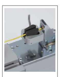
Test image (Crimp terminal tensile test)
