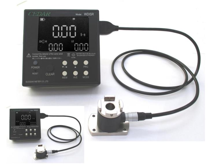
It works with a personal computer or PLC to manage torque measurement more highly. For managing automatic and semi-automatic tools.
