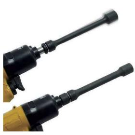
The deepened drive end of the **Sleeve-Drive** tools prevents the sometimes "wobbly" connection between pulse tool - extension - socket. An O-ring inside **Sleeve-Drive** optimizes the perfect fit of extension bars and sockets on the anvil to the effect, that the exactness of the required torque given by the pulse tool is generally improved. Further, the **Sleeve-Drive** avoids the direct transmission of vibrations on the pulse tool and finally on the operator.
