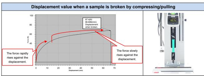
This unit graphs the process and enables you to visually check the force transition until the sample is broken. Also, it helps you to easily find the force/displacement value and peak value when the sample is broken, and leave a comment.
