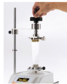
Twist test of screen protective film
