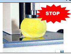
Overload is a condition where a sensor is broken due to excess force applied over its capacity. Once it is overloaded, it requires repair to be able to measure again.
