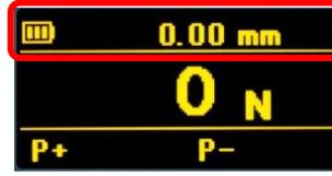
By connecting with a Test-Stand with the linear scale, the displacement value is shown at the display top. It is also possible to output the Displacement Data to a PC by using the available software.
