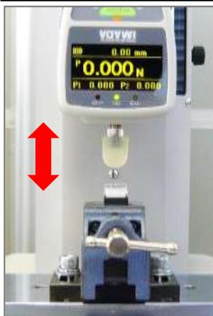
A manual displacement reset is required at the touching sample position.
