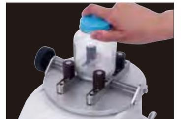
Screw cap opening torque test with DTXS.
