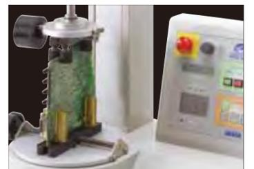
The test example of a circuit board twisting strength test with MTG.
