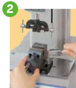
The mounting attachment for the test stand table.
