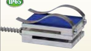
Measuring foot brakes manipulating force by putting the load cell on foot breaks and stepping them together.
