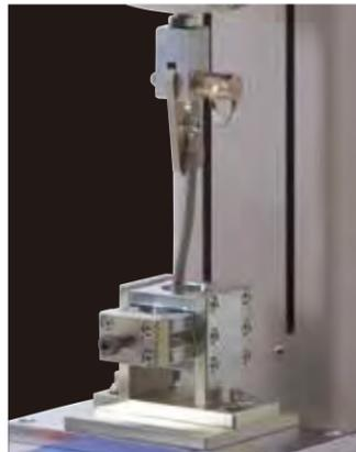
When using CH-5000N and CW-5000N together, the measurement is partly in accordance with JIS C 2805 (2010)
