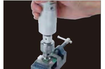
The test example of rotary switch click feeling test with HTGS.
