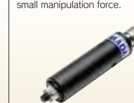
Measure force by mounting each attachment on the thread (the male screw part)
